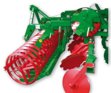
Through the trapezium guide the rollers are directed automatically into the direction of motion.
