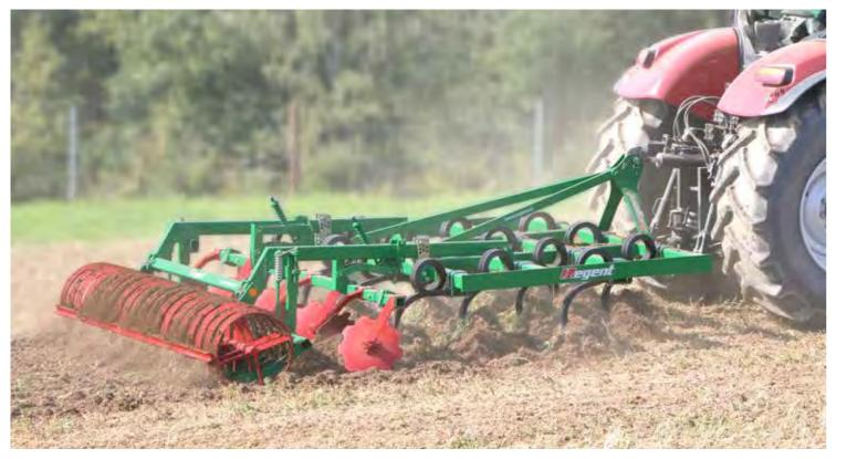
The multifunctional mulch cultivator / chisel cultivator for any field of application - the perfect companion for your fields. Parallelogram suspended discs enable an optimal levelling, furthermore it is infinitely adjustable and overload protected.
